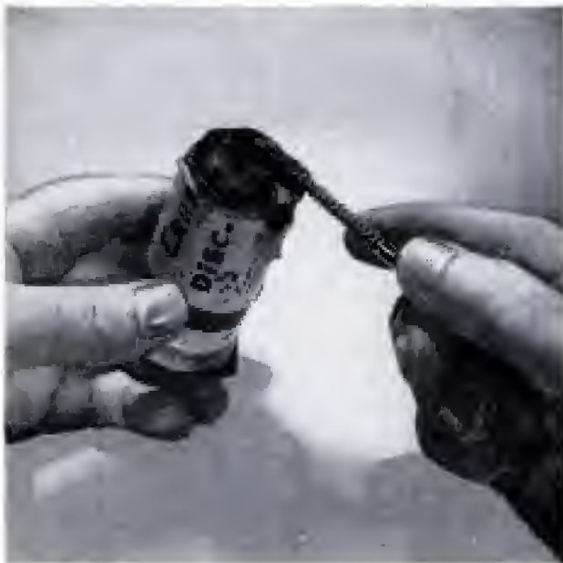
Above, applying cement to the threads of a wood screw eases it into hardwood and at the same time adds to the holding power of the screw. Below, cement applied to face of miter gauge prevents stock from slipping sidewise when making miter cut
